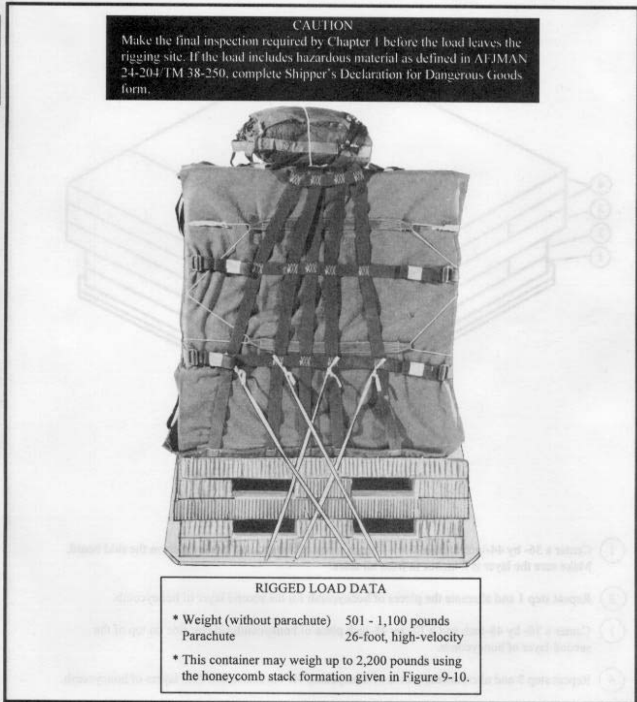
Figure 9-11. A-22 container load weighing less than 1,100 pounds rigged with CVRS for high-velocity airdrop
